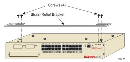
Figure 3-2 Attaching the Strain-Relief Bracket
